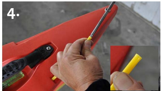
4. When the material has softened by the heating use a large philips screw driver or similar and push into the end of the tube to expand the edge.
