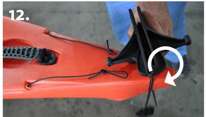
Install the rudder into the Rudder sleeve at the back of the kayak. Make sure the Rudder is turned as much toward the front as possible and turn it.
