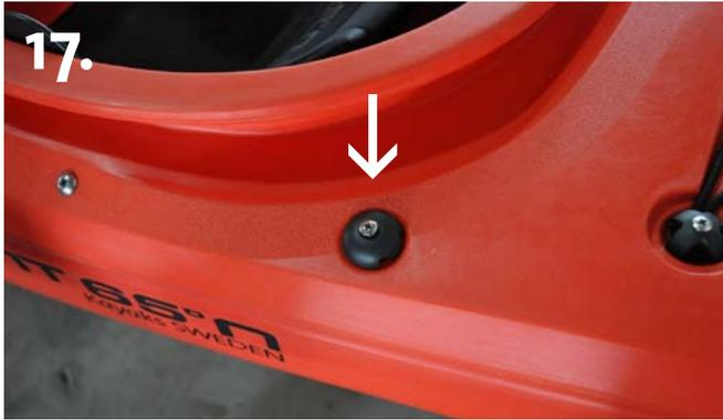
Finally, install the pull up line for the rudder, by first fastening the deck fitting included in the pull up package with the included screw into the insert on the deck
