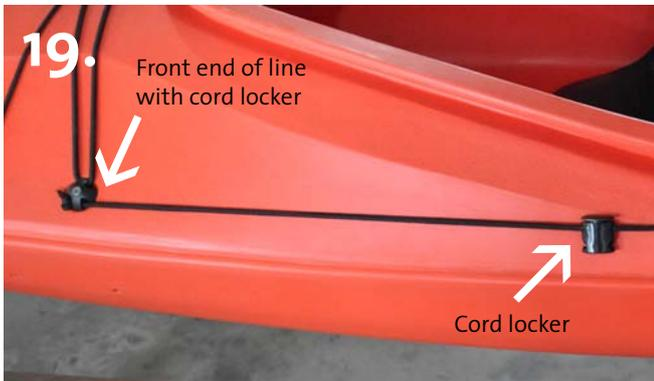
Put the other end of the line with the cord locker into the deck fitting in front of the cockpit. Pull tight and make knot
