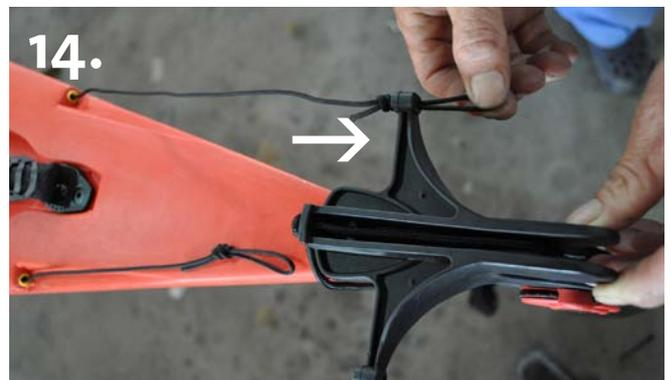
Pull the end of the Rudder line loop through the hole in the rudder "wing". After pulling it through, bend it back over the "wing" and place the end of the loop into the groove above the hole through which it was pulled at
