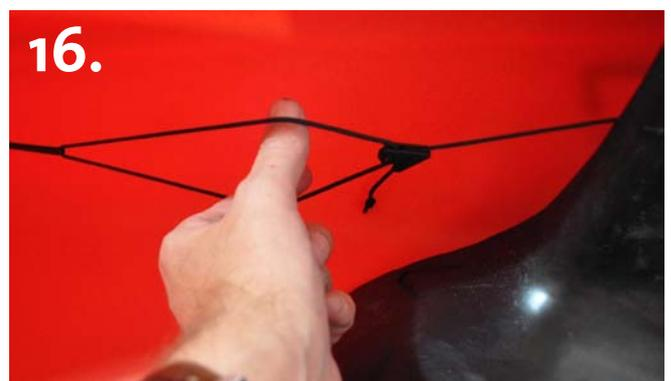
Tighten the rudderlines when sitting in the cockpit by adjusting the mini-line lockers. To tighten, pull the miniliner towards the back. To loosen the lines do as on image above.
