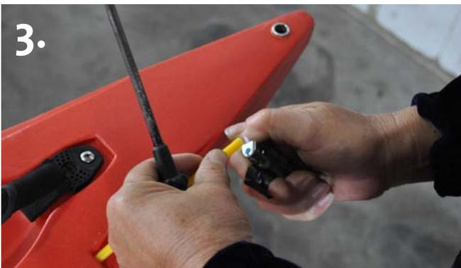
3. Heat the end of the rudder line tube with a butane lighter or similar, but without burning the plastic.
