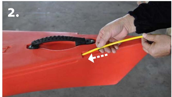
2. Push in the Rudder line tube on each side of the kayak into the holes until approx 15cm remain outside.
