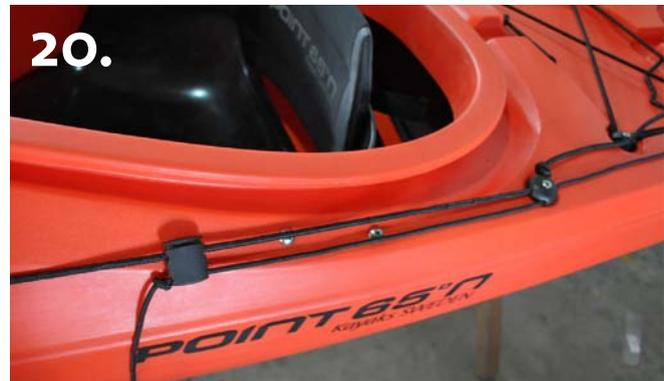
Put the pull up line attached to the rudder through the lower hole in the cordlocker and make a knot to lock it in place. When you have put the cordlocker at a comfortable place where you easily can pull up the rudder by pushing the cord locker forward, you can cut the excess lines and seal the ends with a butane lighter or similar.
