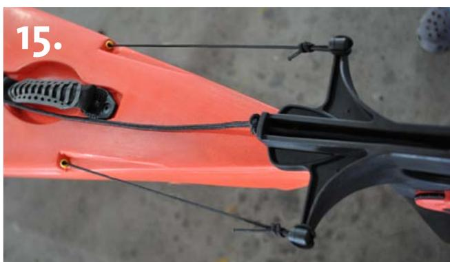
Pull the line tight so to fasten the loop in the groove. With this quick release knot, you can easily dismantle the rudder when transporting the kayak on land.
