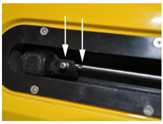
12. Make sure the hole in the metal tube is aligned with the screw and slide the skeg control over it. Screw in the screw into the hole until it grabs the wire and screw tight (not too tight as this can loosen the brass insert in the control). If the brass insert has come loose, send us an e-mail about it, and we will send you a new one.
