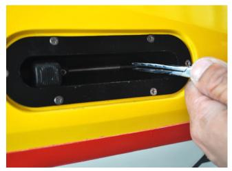
10. Use the thin plyer to grab the wire and guide it into the metal tube
