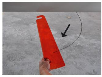
6. Pull out the skeg. If you can't pull it out, the screw on the skeg control is still grabbing the wire – loosen the screw until the skeg is easily pulled out.
