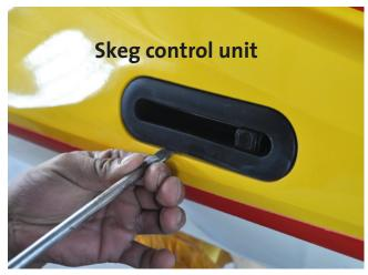
2. Remove the skeg control cover, by carefully inserting the large screwdrivers edge on the outside of the cover. Gently pop it out.
