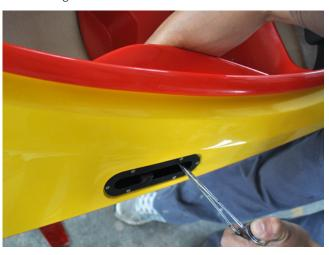
11. You can use your other hand to guide the exposed metal tube steing out inside the cockpit
