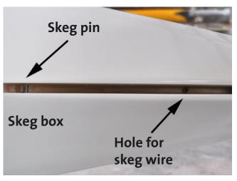
7. Insert the skeg wire into the hole for the skeg wire. When most of the wire is inserted, hook the skeg onto the pin in the skeg box.
