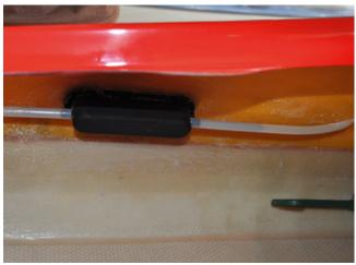
4. Remove the front tube on the skeg control unit so that metal tube is exposed
