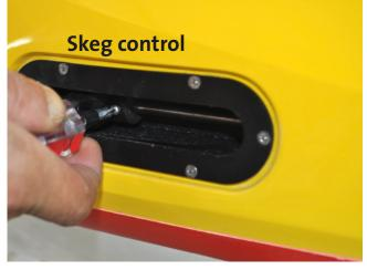
3. Unscrew the skeg control screw which is squeezing the skeg wire. By unscrewing it the skeg wire will be loosened.
