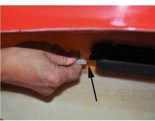
9. If the skeg wire is difficult to steer into the skeg control unit, gently loosenthe plastic tube at the back of the control unit, and guide the wire into the hole
