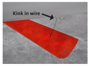
The wire in the skeg can kink easily if the kayak is set down on the ground or beached with the skeg deployed. This will make it very difficult or even impossible to pull the skeg up or down with the skeg control unit, as the wire will simply fold on itself inside the skeg box.
