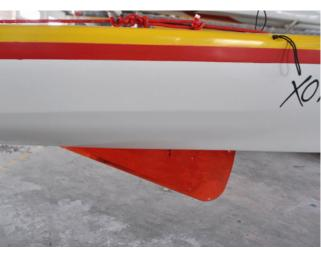
13. Make sure skeg does not come out to far when the control is pushed all the way back
