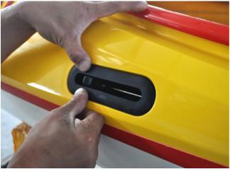
17. Put back the skeg sontrol unit cover by gently pushing the inside edge over the lip inside the unit
