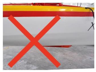
16. If the skeg doesn't go all the way into the skeg box, re-adjust after loosening the screw on the skeg control.
