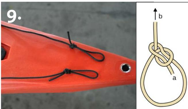
9. Make a Bowline knot at the end of the rudder lines (see image). The loop should be approx 3cm at the end. Heat the ends of the lines with a butane lighter to seal the line ends.
