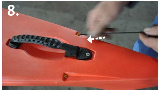
8. Push the Rudder line through the tube until it appears at the other end inside the cockpit. Sometimes this can be difficult as the line might bunch up inside the tube, if this happens, you can use a thin steel wire first on which you attach the rudderline to pull it with.
