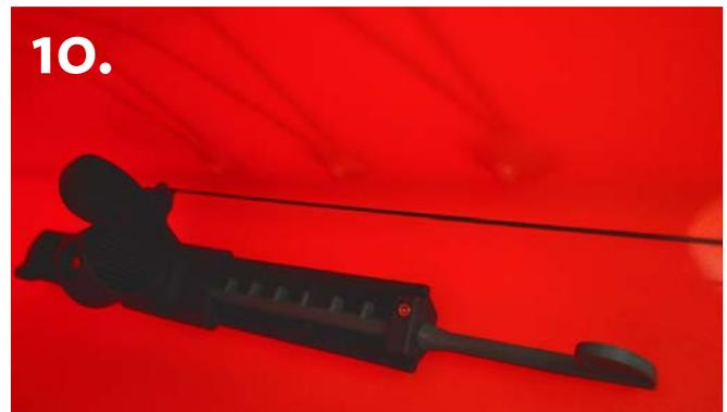
10. The foot rests are easily replaced with the rudder pedals by unscrewing the 6mm screws from the outside. It will be easier to put in the pedals if you get some help in holding the pedal on the inside while. The pedals are clearly marked with "L" for Left and "R" for Right.
