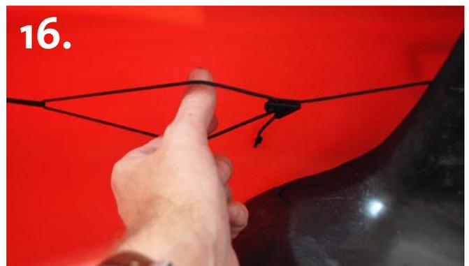
Tighten the rudderlines when sitting in the cockpit by adjusting the mini-line lockers. To tighten, pull the miniliner locker towards the back. To loosen the lines do as on image above.
